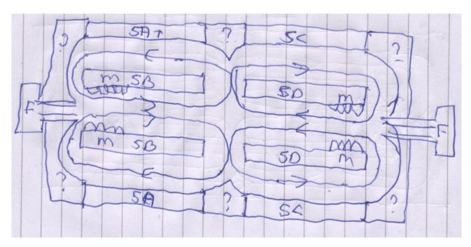
This is my version of Not A Large Hadron Collider. OK. In effect it is two storage rings comprising a pair of concentric solenoids [SA-SD] along with some ? Things to direct the beams around the bendy bits. Maintenance accelerators, M, and fuelling accelerators, F. The arrowed lines are the paths of our nucleons with their Kissing points.
